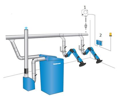
Airflow alarm and pressure switch mounted
