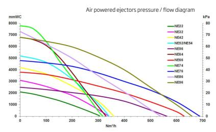
Air Powered ejectors
