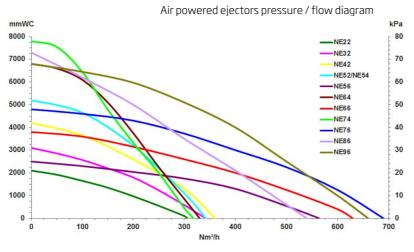
Air Powered ejectors
